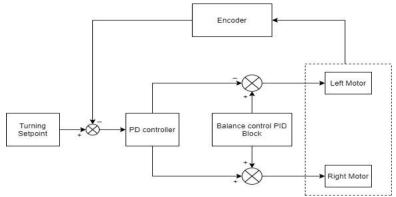
Fig. 6. PD control for turning motion
