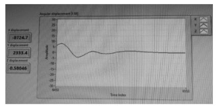
Fig. 11. PID Response of system to Disturbance
