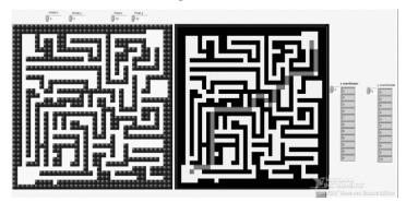
Fig. 12. End result of the A\* path planning algorithm
