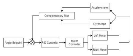
Fig. 4. PID control for self-balancing
