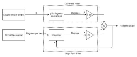
Fig. 3. Block Diagram of Complementary filter
