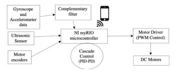
Fig. 1. Block Diagram of the Robot
