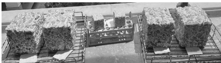
Fig. 14. Degraded concrete and mortar cubes after acid attack
