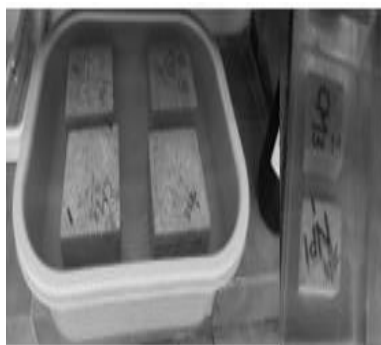
Fig. 7. Concrete and mortar cubes immersed in the 5% sulfuric acid solution
