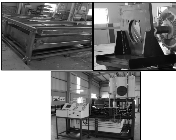
Fig. 2. a) Base frame, b) L Bracket Assembly, c) Fabricated model of hydraulic pump test rig
