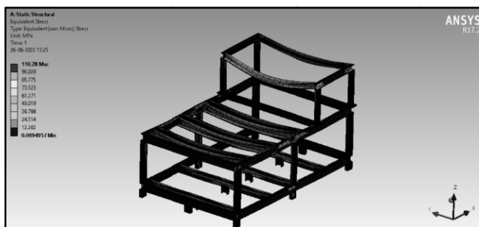
Fig. 4. a) Total deformation and b) Equivalent Von mises stress of base frame
