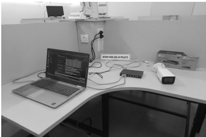
Fig. 2. Receiving live video feed by connecting CCTV camera with laptop
