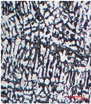
As cast (a) Microstructure 100X
