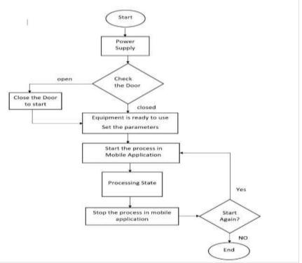
Fig. 7. Workflow of the Equipment
