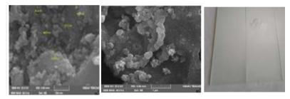
Fig. 9. SEM images of the ZnO films prepared and image of coating on glass.
