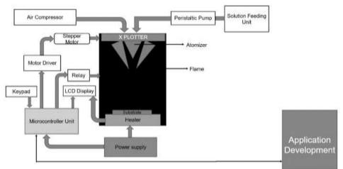
Fig. 1. Schematic representation of Spray pyrolysis system
