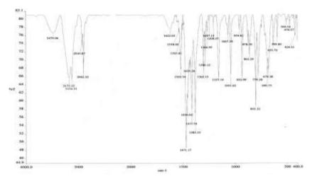
Fig. 1. FT IR spectrum (in KBr) of CuLCl2
