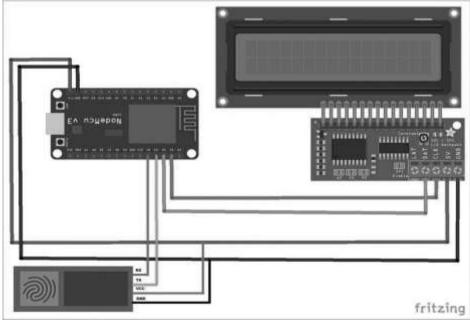
Fig. 2. Fritzing Diagram of Biometric module
