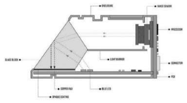
Fig. 1. Schematic of R307 Fingerprint Sensor
