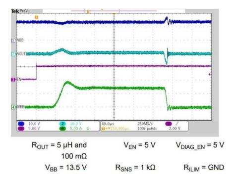
Fig. 10. IVBB With RILIM Shorted to Ground
