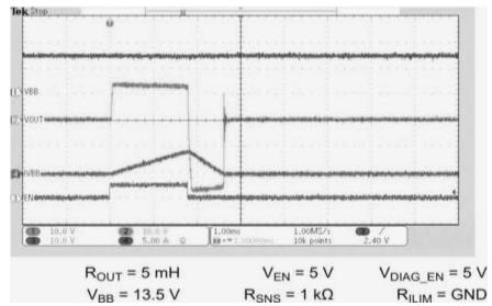
Fig. 9. 5mH Inductive Load Driving
