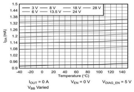
Fig. 13. Diagnostic Current IDIAG vs Temperature
