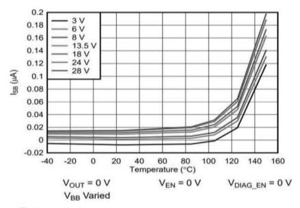
Fig. 11. Standby Current I<sub>sb</sub> vs Temperature
