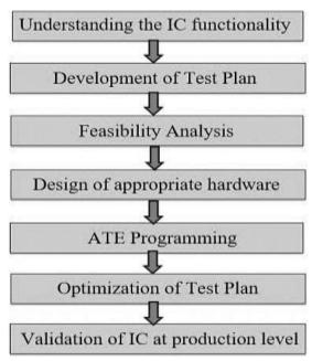
Fig. 2. I C Testing Methodology Flowchart
