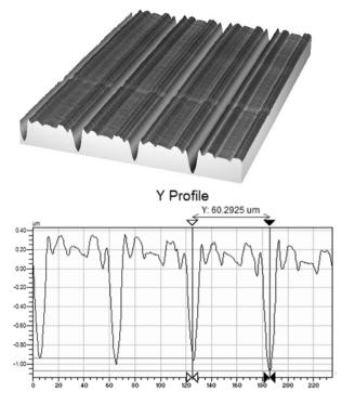
Fig. 3. a). Surface topography and b). Cross sectional profile of texture L2
