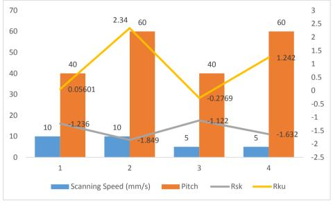
Fig. 4. Effect of scanning speed and Pitch on R<sub>sk</sub> and R<sub>ku</sub>
