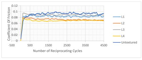
Fig. 6. Friction performance of textured and untextured specimen
