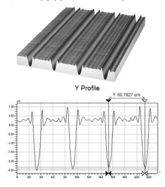
**Fig. 5. a**). Surface topography and **b**). Cross sectional profile of texture L4 RVJSTEAM, 1,2 (2020)
