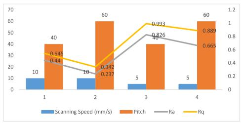
Fig. 3. Effect of scanning speed and pitch on Ra and Rq
