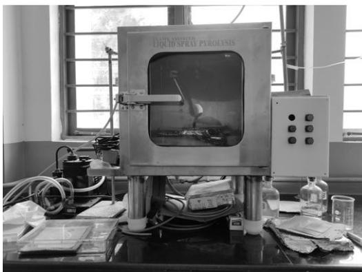
**Fig. 4.** Flame assisted liquid Spray pyrolysis chamber
