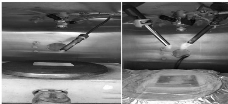
**Fig. 3.** Single and double flame unit fitted next to spray nozzle inside the chamber
