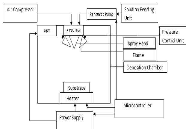
**Fig. 1.** Schematic representation of Spray pyrolysis system
