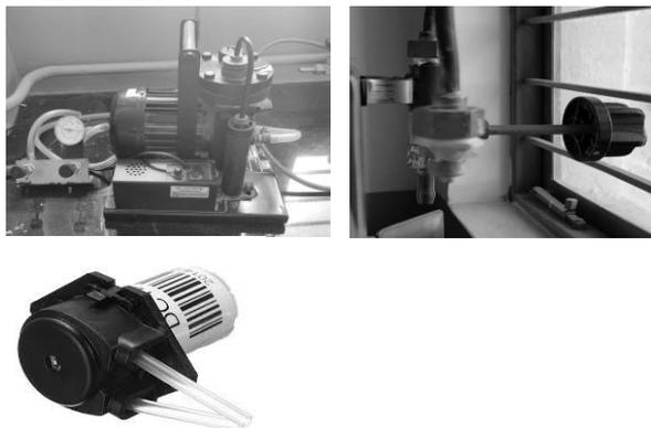
**Fig. 2.** Air compressor, gas control and peristaltic pump
