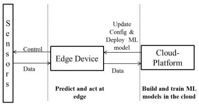
Fig. 5. Edge Intelligence with Cloud-based IoT
