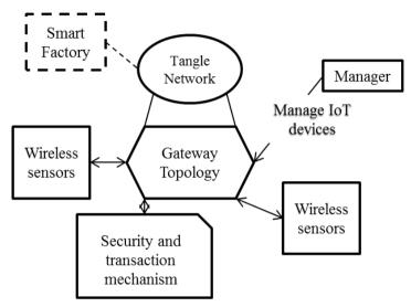
Fig. 8. Blockchain-based IIoT for smart factory
