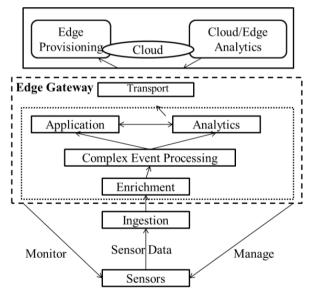
Fig. 4. Edge Intelligence and IoT Sensor Stream System
