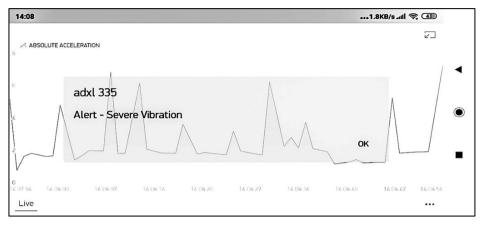
Fig. 11. Real time Absolute acceleration graph with alert notification (case 3)
